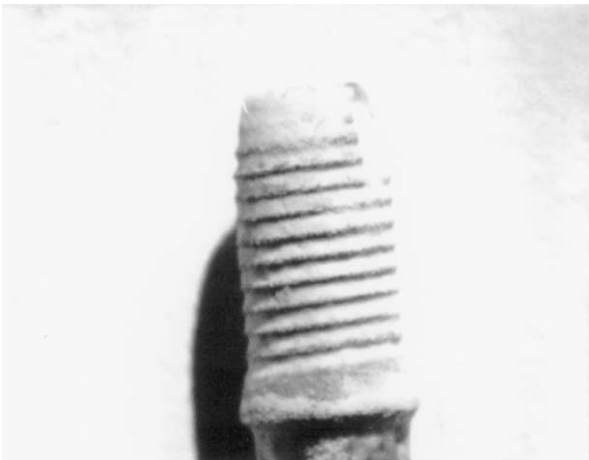
Fig. 8. General view of the threaded screw coated by the optimised two-step firing process.
